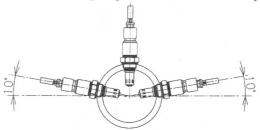
After welding the sensor boss to the exhaust, run an M18 x 1.5mm tap or thread cleaner (KD Tool P/N 730 or equivalent) through the boss to remove any thread-distortion. If this is not done, the sensor's threads may be damaged during installation or removal. Apply a small amount of anti-seize compound to the threads and tighten the sensor to 45~55N·m (Previously stated as 1/2~2/3 turn)
