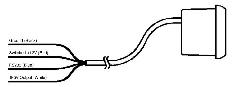
Figure 1. Connection Diagram
